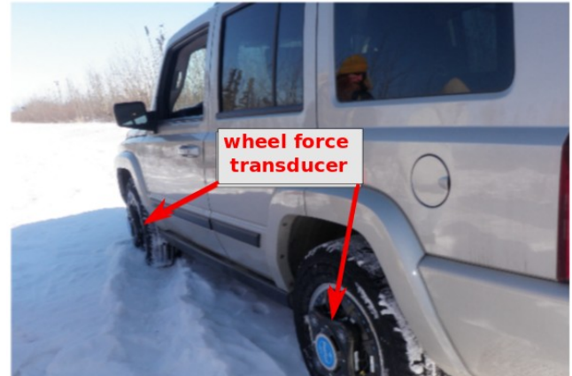
Figure 3: Instrumented ground vehicle.
